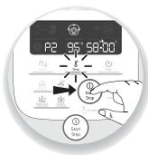
3- When you have finished entering all your settings, press the “start” button **(B5)**. When your appliance is using cooking mode, the red indicator light, lights up to inform you that cooking has started. When the program has started, you have the possibility of stopping the appliance at any time by pressing the “stop” button **(B5)**.
