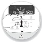
2- The pre-programmed settings can be modified for the time of a recipe (depending on the chosen recipe, ingredients and quantities prepared). Press the cooking temperature selector (B2) or the time selector (B3): the chosen setting will flash on the screen (C6-C7).
