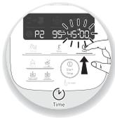
1- Press directly on the button for the setting you want to adjust, i.e. the speed selector **(B1)** or the cooking temperature selector **(B2)** or the time selector **(B3)**, the chosen parameter flashes on the screen **(C5-C6-C7)**.
