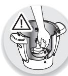
Take care with the knives of the Ultrablade knife (F1) and the kneading & grinding blade (F4) when you are cleaning them and when you empty the bowl, they are extremely sharp. Be careful if a hot liquid is poured into the food processor because it could be ejected from the appliance due to it suddenly boiling.
